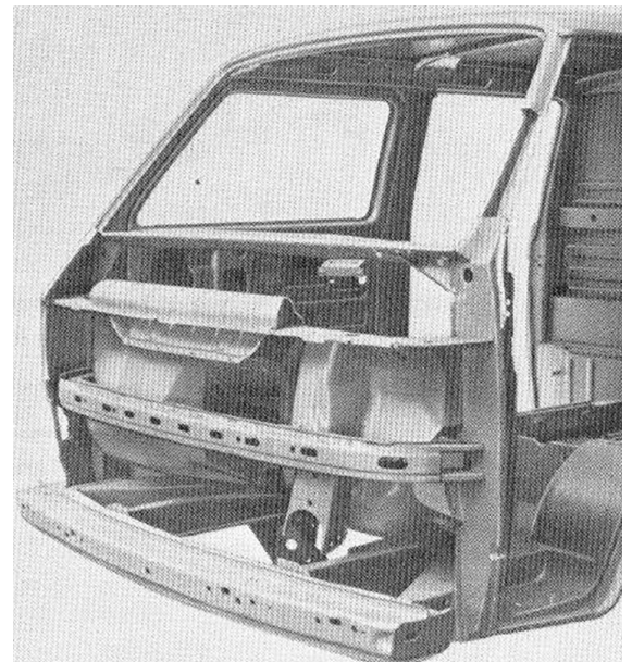
Fig. 5: Front panel corner section — part section and front aprons
